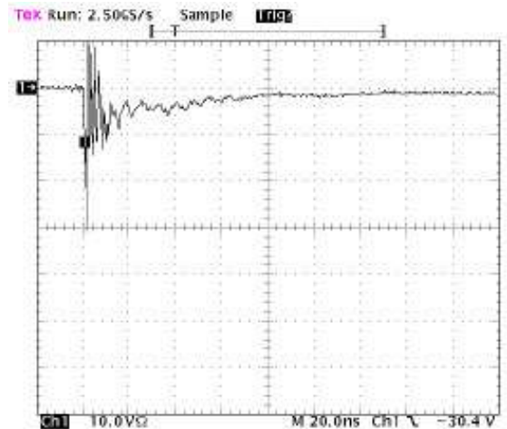
Figure 3. ESD Clamping Voltage Screenshot Negative 8 kV Contact per IEC61000-4-2
